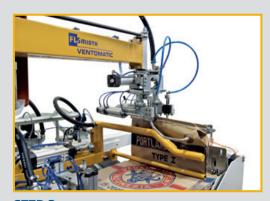
**STEP 3 Valve opening**The valve is opened by the suction discs, during the transport towards the spout.
