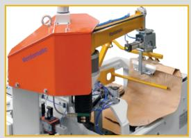
STEP 3 Clamping and valve opening
