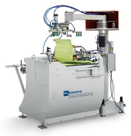
INFILROT® BU SB HDPE mechanical arm bag applicator for stitched HDPE plastic bags
